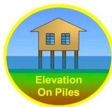
**2) Elevating the Building.** This involves moving the structure up and increasing the elevation of the floor. This can be done using fill, although many buildings may also be elevated with extended concrete walls or columns, piers and piles. Buildings that are slab-on-grade would be handled differently than walk-out basements (see below).
