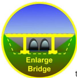
**Bridge Raises** are a form of a bridge enhancement and are vertical improvements to improve the area of flow, similar to **Bridge Widening**, although a raise will also require elevating the profile of the road and involve more costs.
