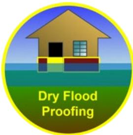
**Dry Flood Proofing** is a physical **Nonstructural Measure** for **Flood Proofing** structures in the floodplain and involves sealing building walls with waterproofing compounds, impermeable sheeting, or other materials to prevent the entry of floodwaters into damageable structures. Dry flood proofing is applicable in areas of shallow, low velocity flooding.
