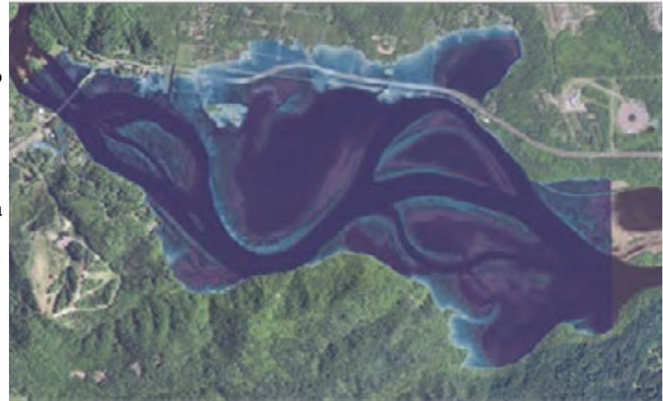
An inundation map showing approximate flood-peak extents and depths for June 2012 on St. Louis River in Duluth, MN. (Map prepared by C. Czuba, USGS, Nov 2012. Map based from 2010 National Agricultural Imagery program.)
